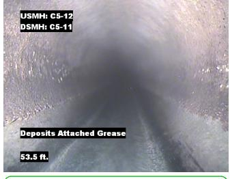
**Distance**: 53.5 ft. **Grade**: 2 **Condition**: Deposits Attached Grease
