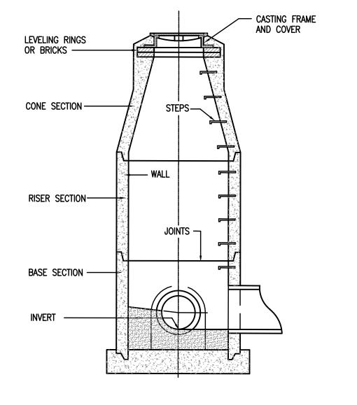
MANHOLE COMPONENTS DETAIL
