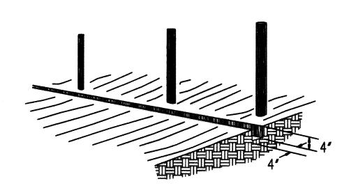
. SET POSTS AND EXCAVATE A 4"X4" TRENCH UPSLOPE ALONG THE LINE OF POSTS
