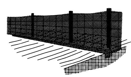
4. BACKFILL AND COMPACT THE EXCAVATED SOIL
