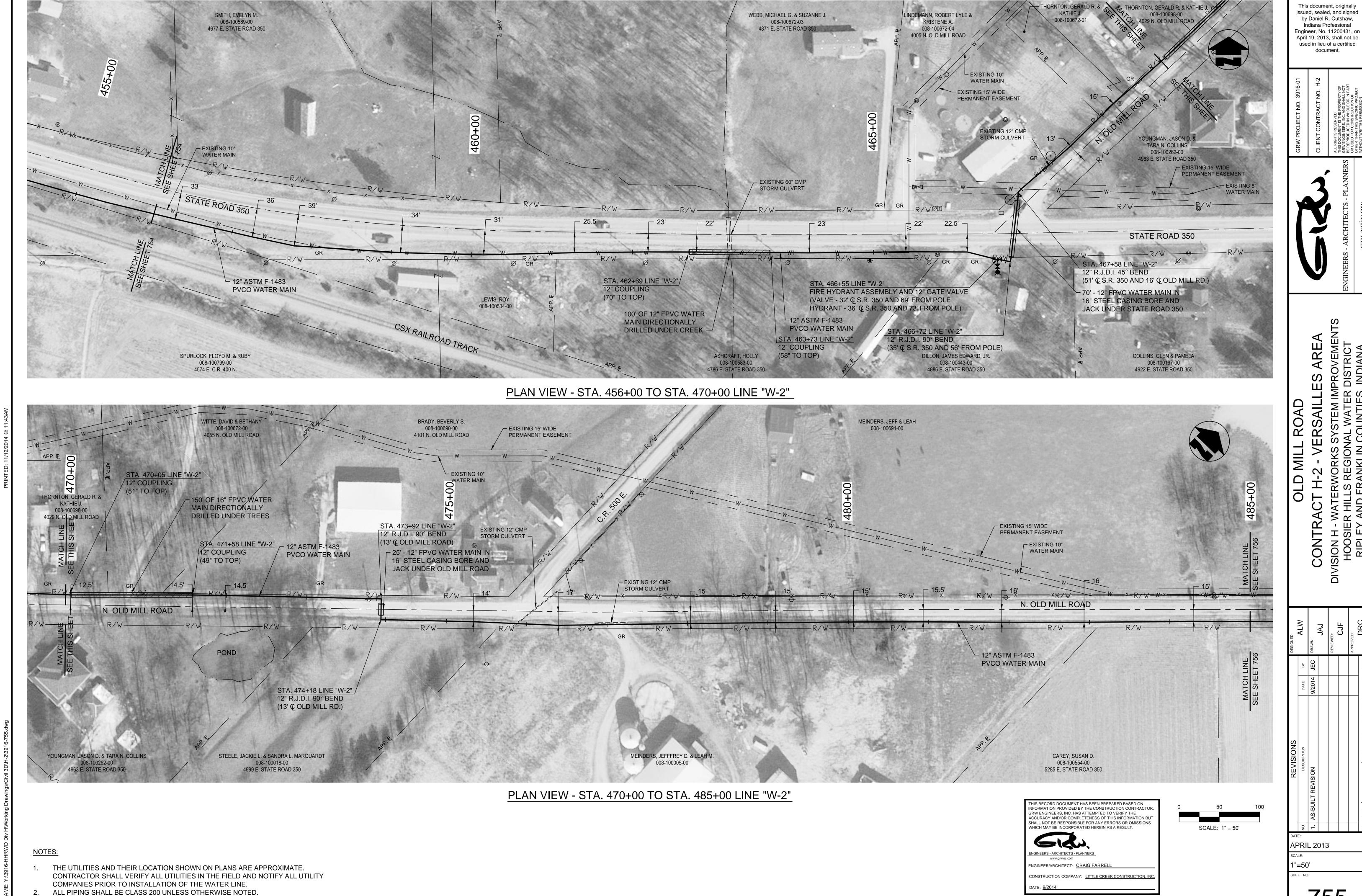
48" MINIMUM COVER REQUIRED OVER TOP OF WATER LINE UNLESS OTHERWISE NOTED.
