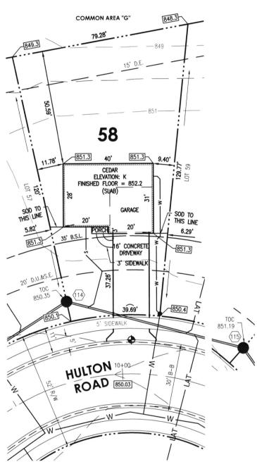
NOTE: THE FOOTINGS FOR THIS HOUSE SHOULD BE PINNED SINCE THERE IS LITTLE TOLERANCE FROM THE 5' SIDE YARD SETBACK, CALL US WHEN FOOTING IS IN SO WE CAN SCHEDULE PINNING
