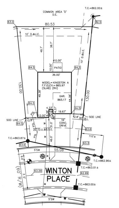
PROPOSED GRADE PER PLAN XX.XAB AS BUILT GRADE S.S.D. SUB-SURFACE DRAIN SANITARY SEWER ASI 6" AS BUILT SANITARY LATERAL
