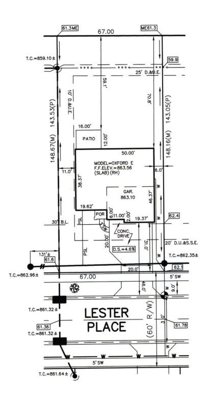
LEGEND: PROPOSED GRADE PER PLAN XX.XAB AS BUILT GRADE S.S.D. SUB-SURFACE DRAIN SANITARY SEWER
