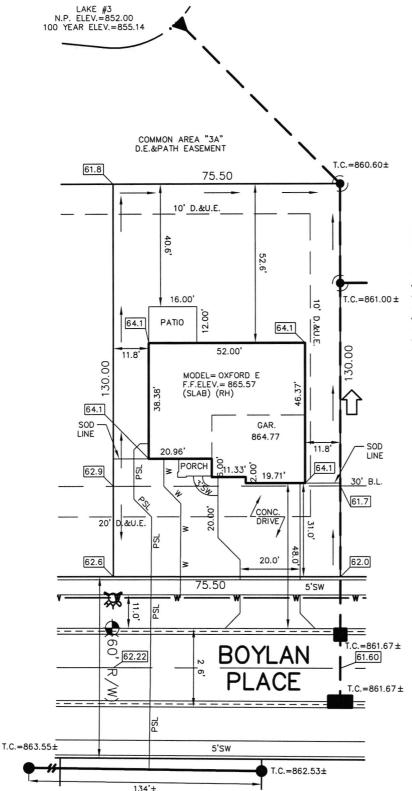
PROPOSED GRADE PER PLAN XX.X XX.XAB AS BUILT GRADE S.S.D. SUB-SURFACE DRAIN SANITARY SEWER PSL
