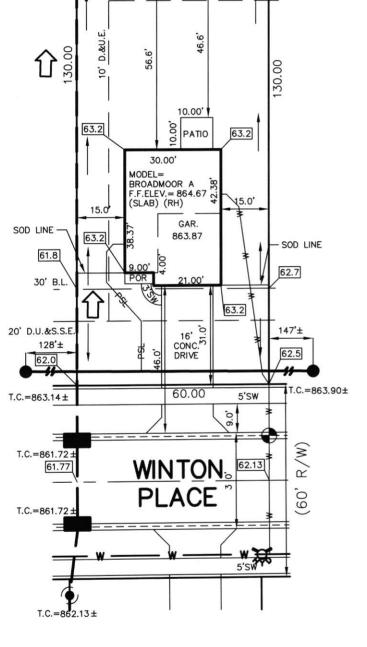
WATER MAIN 3/4" WATER CONNECTION SWALE SANITARY MANHOLE STORM MANHOLE CURB INLET FIRE HYDRANT STREET TREES EMERGENCY FLOOD ROUTE DRAINAGE, UTILITY & SANITARY SEWER EASEMENT D.U.&S.S.E.
