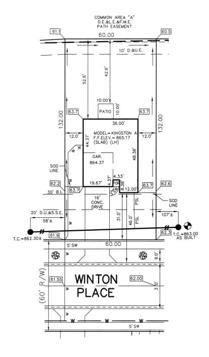
LEGEND: PROPOSED GRADE PER PLAN XX.XAB AS BUILT GRADE <u>S.S.D.</u> SUB-SURFACE DRAIN SANITARY SEWER 6" AS BUILT SANITARY LATERAL 6" PROPOSED SANITARY LATERAL ASL PSL STORM SEWER
