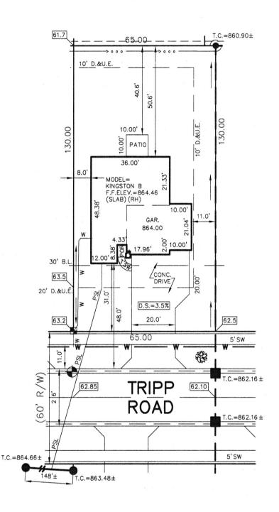
LEGEND: PROPOSED GRADE PER PLAN XX.XAB AS BUILT GRADE S.S.D. SUB-SURFACE DRAIN SANITARY SEWER ASL 6" AS BUILT SANITARY LATERAL 6" PROPOSED SANITARY LATERAL STORM SEWER 3/4" WATER CONNECTION WATER MAIN W SWALE SANITARY MANHOLE STORM MANHOLE CURB INLET FIRE HYDRANT STREET TREE WATER METER DRAINAGE & UTILITY EASEMENT BUILDING LINE MINIMUM FINISHED FLOOR ELEVATION MINIMUM FLOOD PROTECTION GRADE D.&U.E. B.L. M.F.F.E. M.F.P.G.
