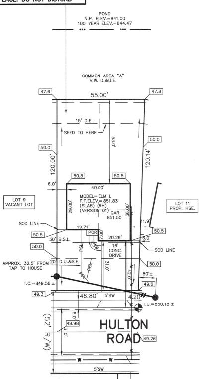
CONTRACTOR SHALL CUT 13.5' OFF OF LATERAL AND BEGIN FROM THAT POINT AND CONNECT TO HOUSE FOLLOWING PLOT PLAN.
