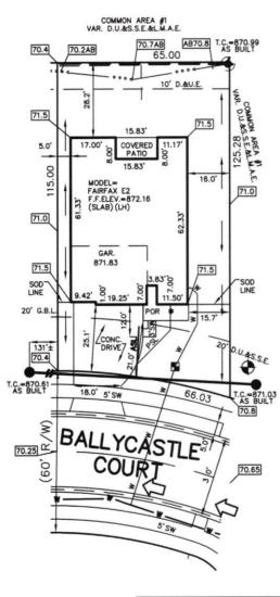
CONTRACTOR SHALL CUT 14' OFF OF LATERAL AND BEGIN FROM THAT POINT AND CONNECT TO HOUSE FOLLOWING PLOT PLAN.
