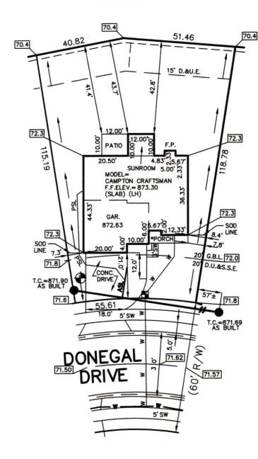
CONTRACTOR SHALL CUT 6' OFF OF LATERAL AND BEGIN FROM THAT POINT AND CONNECT TO HOUSE FOLLOWING PLOT PLAN.
