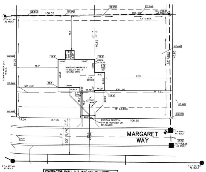
CONTRACTOR SHALL CUT 15.0' OFF OF LATERAL AND BEGIN FROM THAT POINT AND CONNECT TO HOUSE FOLLOWING PLOT PLAN.
