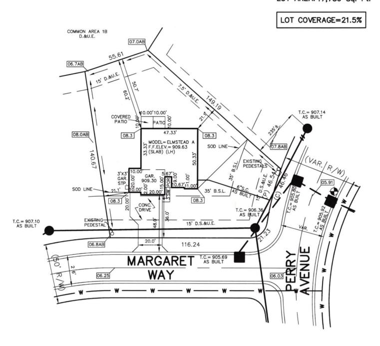
ALL UNDERGROUND SEWERS AND UTILITIES SHOWN ARE PLOTTED BY SCALE FROM "RECORD DRAWINGS" FURNISHED BY ENGINEER.
