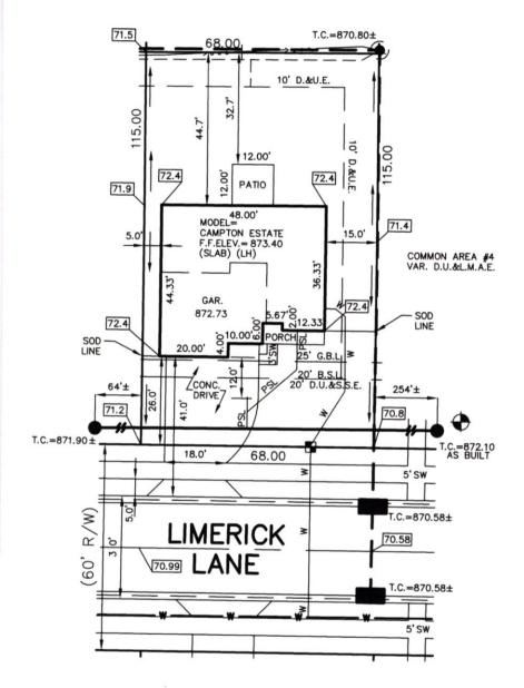
CONTRACTOR SHALL CUT 4.5' OFF OF LATERAL AND BEGIN FROM THAT POINT AND CONNECT TO HOUSE FOLLOWING PLOT PLAN.
