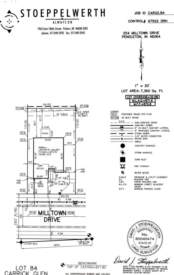
BENCHMARK TOP OF CASTING=871.80 ALL UNDERGROUND SEWERS AND UTILITIES SHOWN ARE PLOTTED BY SCALE FROM DESIGN PLANS FURNISHED BY ENGINEER THE ACTUAL FIELD LOCATION MAY VARY.
