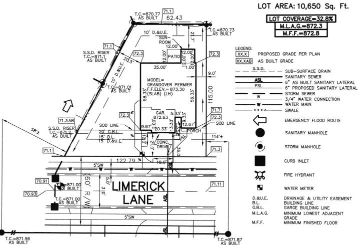
CONTRACTOR SHALL CUT 8' OFF OF LATERAL AND BEGIN FROM THAT POINT AND CONNECT TO HOUSE FOLLOWING PLOT PLAN.
