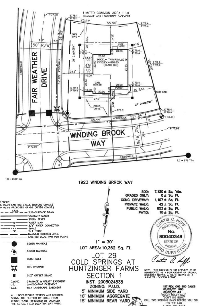
ALL UNDERGROUND SEWERS AND UTILITIES SHOWN ARE PLOTTED BY SCALE FROM DESIGN PLANS FURNISHED BY ENGINEER THE ACTUAL FIELD LOCATION MAY VARY.
