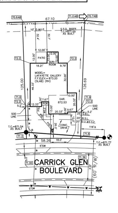
PROPOSED GRADE PER PLAN XX.X XX.XAB AS BUILT GRADE S.S.D. SUB-SURFACE DRAIN SANITARY SEWER 6" AS BUILT SANITARY LATERAL 6" PROPOSED SANITARY LATERAL PSL STORM SEWER 3/4" WATER CONNECTION WATER MAIN W W SWALE SANITARY MANHOLE STORM MANHOLE CURB INLET FIRE HYDRANT WATER METER EMERGENCY FLOOD ROUTE DRAINAGE, UTILITY & SANITARY
