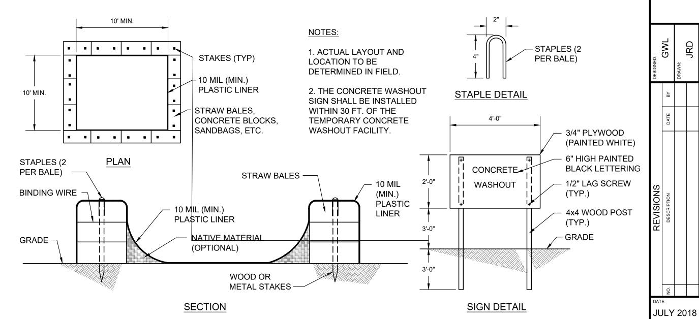
**CONCRETE WASHOUT DETAILS** NOT TO SCALE
