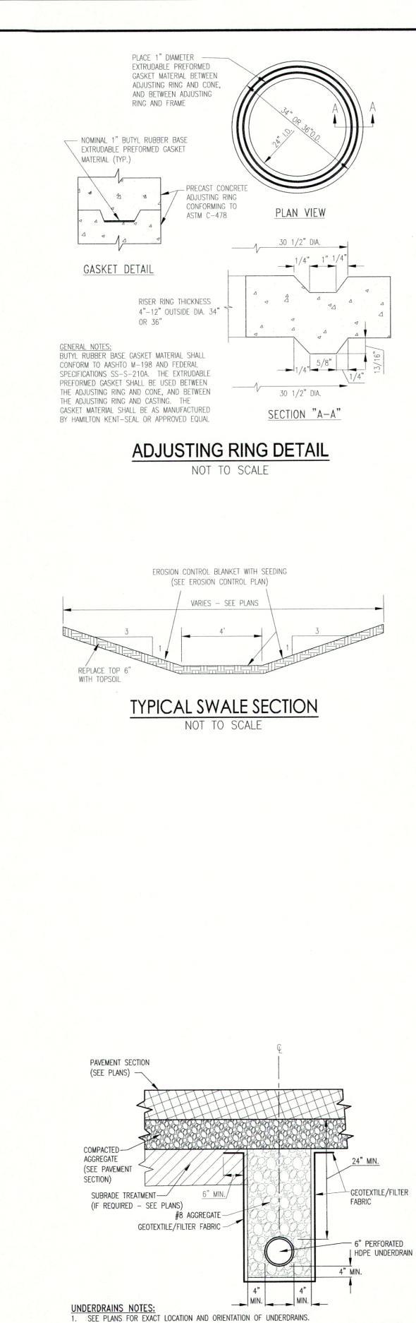
UNDERDRAIN GRADES SHALL NOT BE LESS THAN 0.30% AND THE PIPE SHALL BE DISCHARGED INTO
