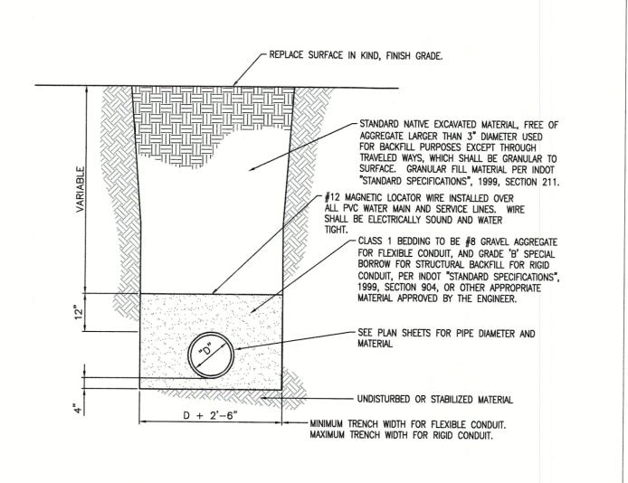
STANDARD WATER PIPE TRENCH & BEDDING DETAIL
