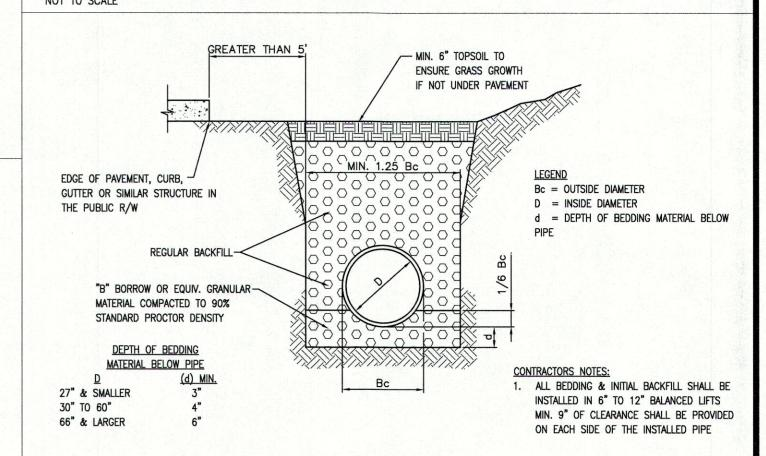
REINFORCED CONCRETE PIPE (RCP) TRENCH DETAIL GREATER 5' FROM EDGE OF PAVEMENT NOT TO SCALE
