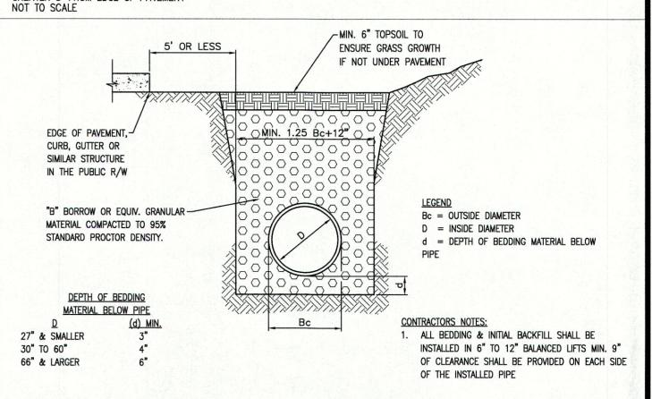
REINFORCED CONCRETE PIPE (RCP) TRENCH DETAIL WITHIN 5' FROM EDGE OF PAVEMENT NOT TO SCALE
