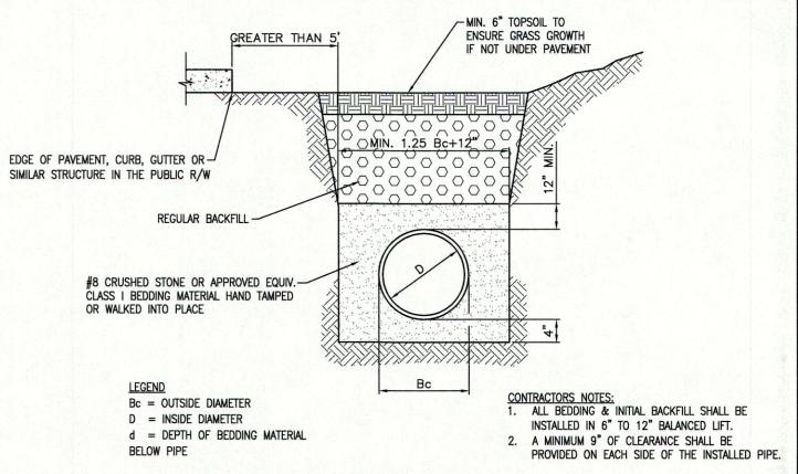
PLASTIC PIPE (PVC & HDPE) TRENCH DETAIL GREATER 5' FROM EDGE OF PAVEMENT NOT TO SCALE
