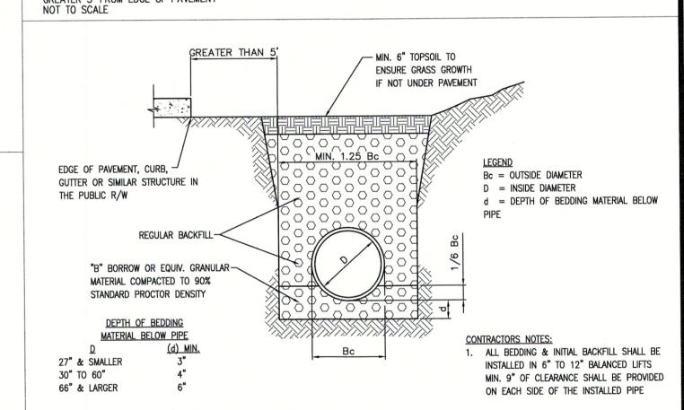
REINFORCED CONCRETE PIPE (RCP) TRENCH DETAIL
