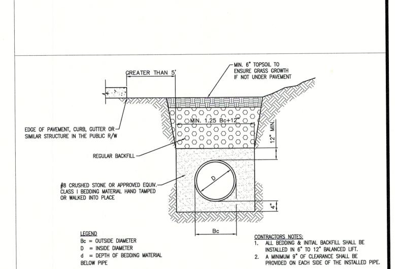
PLASTIC PIPE (PVC & HDPE) TRENCH DETAIL
