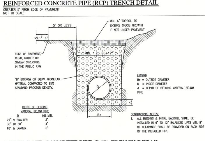
REINFORCED CONCRETE PIPE (RCP) TRENCH DETAIL WITHIN 5' FROM EDGE OF PAVEMENT NOT TO SCALE
